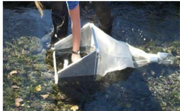
A Suber Sampler is used to collect macroinvertebrates from the river bed. The river bottom is agitated and rocks scrubbed within the 25x25cm square. Invertebrates collect in the net. Three to five replicates will be taken at each site.
