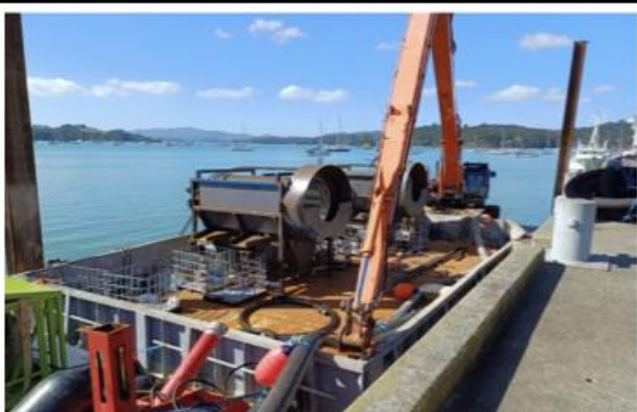
Barge with suction head and 2 large trommels to separate the Caulerpa as it's sucked from the seabed
